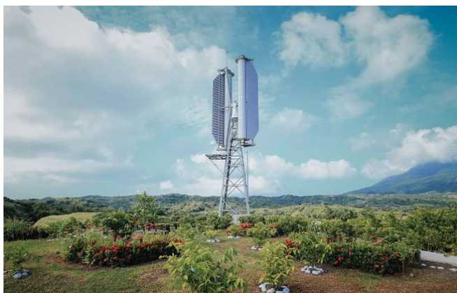
Example of a Flagship Project Microgrids with magnus windmills In the Republic of the Philippines
